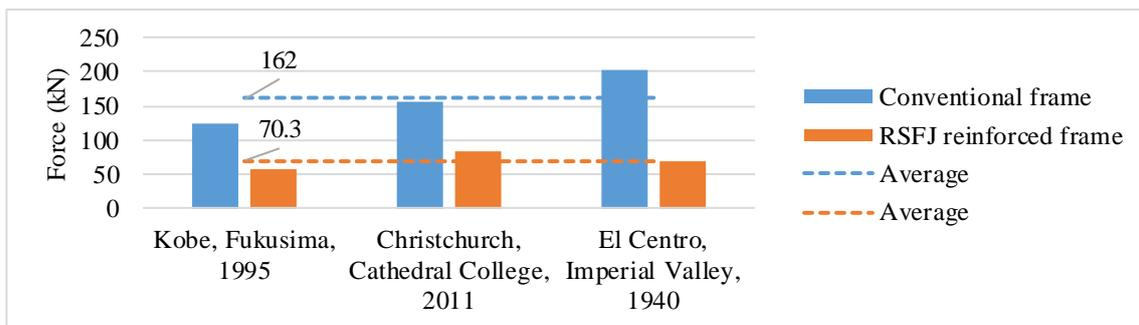
Figure 8. Comparison of maximum base shears under the scaled earthquakes and their average
