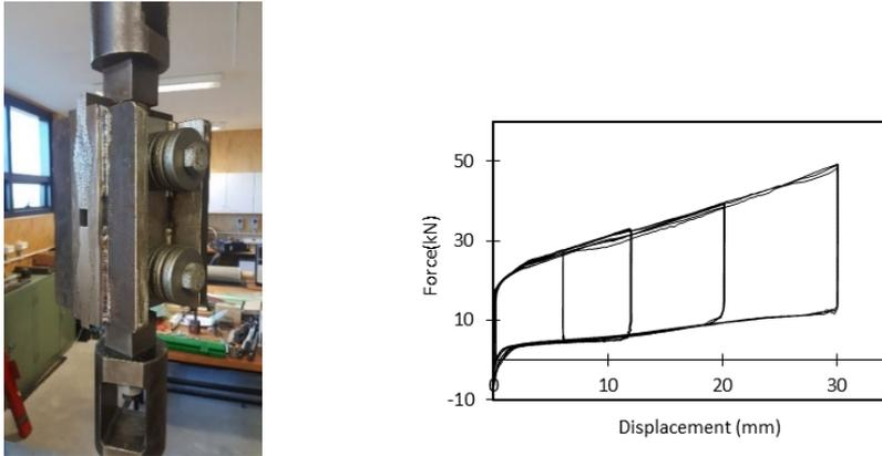
Figure 5. Joint component testing of the RSFJ [11]
