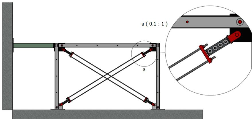
Figure 6. The designed test set-up
