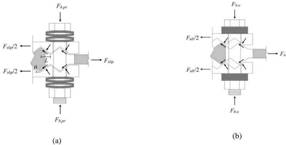
Figure 3. Free body diagram of the RSFJ at (a) slip state, (b) ultimate state [11]
