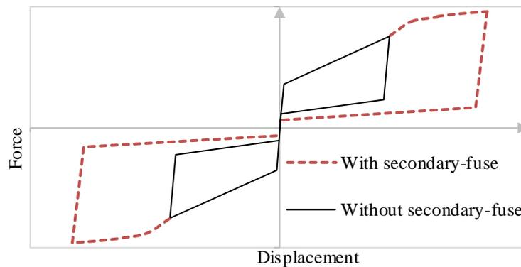
Figure 4. Flag-shape response of the RSFJ with and without the secondary-fuse mechanism
