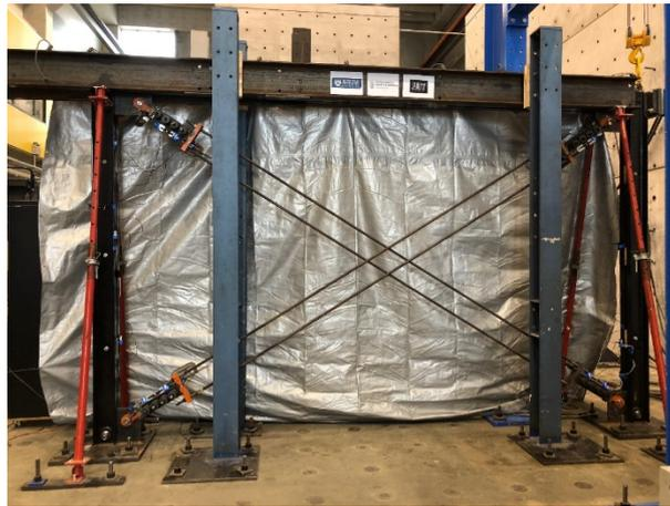
Figure 11. The erected main frame and the protection frame ready to be tested
