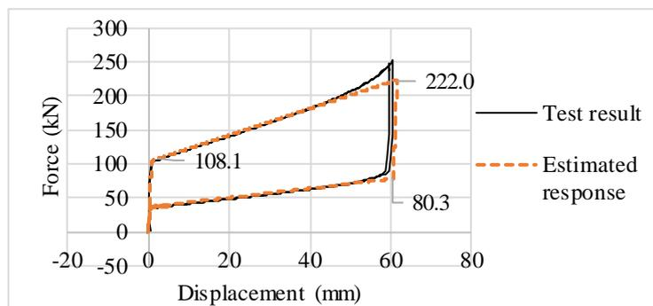
Figure 10. Comparison of the joint component test result and the estimated response
