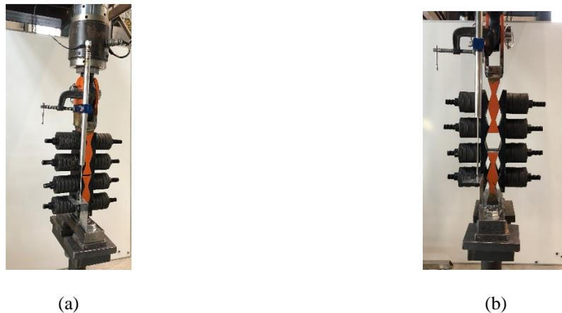
Figure 9. RSFJ component testing: (a) setup, (b) RSFJ at the maximum designed displacement (60 mm)
